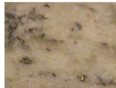
Cut slab of Coleman core showing visible gold. Previous metallurgical test work indicates +80% gold recoveries with simple gravity processing.
