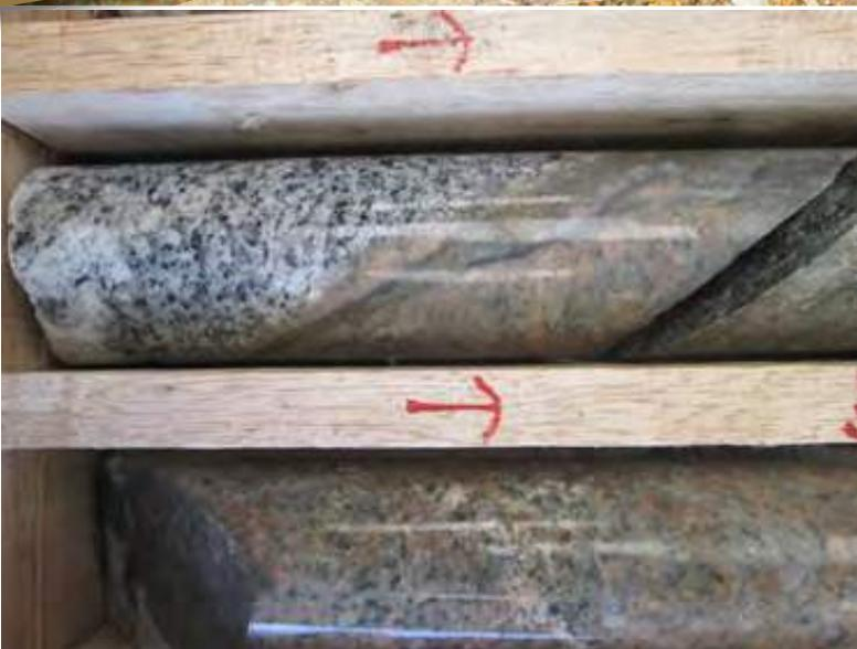
**Drill core from Gramalote showing the quartz-pyrite-gold veinlets that cut through the granite.**
