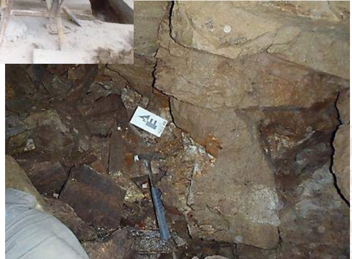
0.2m mineralized structure inside Lyra. Qz, FeOx, Galena, S40E/30SW. 0.2m@34g/tAu-19.65g/tAg-0.85%Pb
