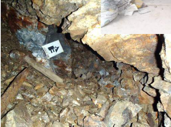
0.6m mineralized structure inside Lyra. Qz, FeOx, Galena, N20E/30SE. 0.6m@70g/tAu-26.6g/tAg-0.86%Pb
